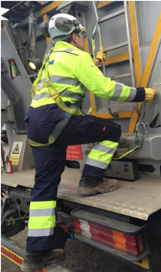
Figure 8.3: Examples of accessing the machine utilising collective and personal fall protection system
